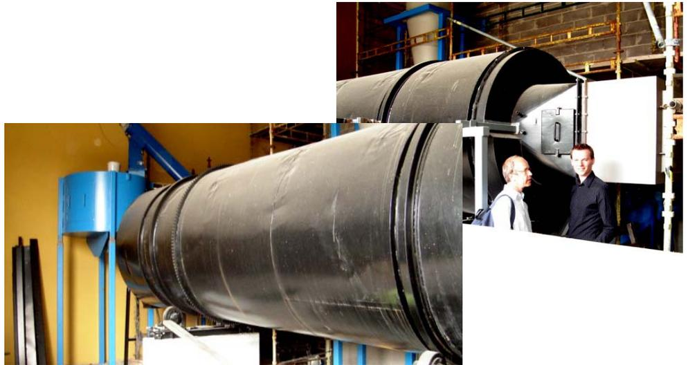
A rotary drum dryer uses an existing off-gas from the sawmill's energy plant consisting of a furnace and a boiler. The sawmill uses only dry chips as fuel, which implies that the off-gas has a very high drying potential.
