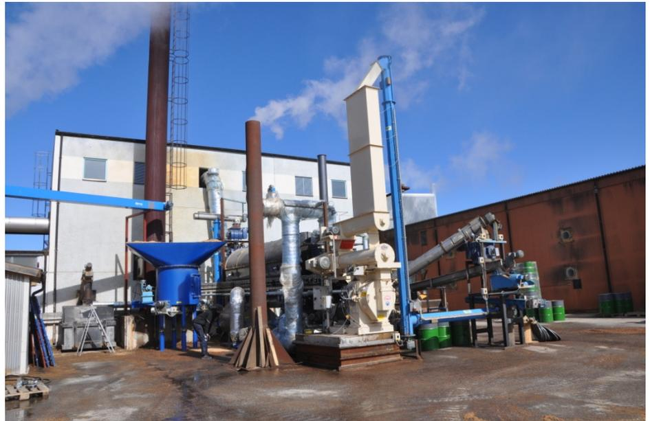
The Torrefaction process takes place in a rotary, tubular reactor which is heated indirectly with flue gases from a biosolids furnace. The flue gas is recovered at two different temperatures, approx. 350 °C and 800 °C. The flue gas is mixed in a mixing chamber with a part of the outgoing flue gases from the reactor in order to reach the required temperature.
