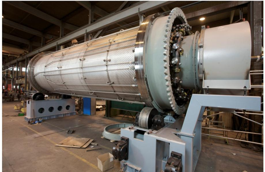
The cooling of the material is executed in two parallel rotating tubular coolers. The tubulars are indirectly cooled by water through the mantel surfaces and tubes inside the rotor.
