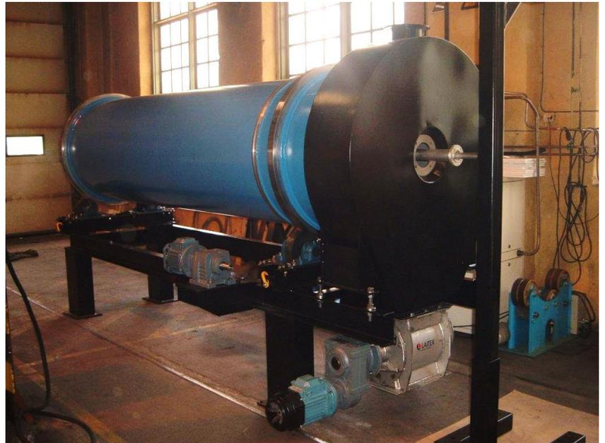
Dewatered Tellurium concentrate is delivered in batches to the dryer from a mechanical press filter through a material handling system equipped with load cells to ensure an even feeding rate of the material into the dryer.
