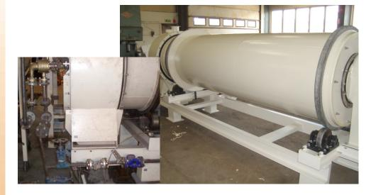
A rotary dryer, in this case heated with 3 bar steam from the grid, dries this very sticky and temperature sensitive material after a mechanical dewatering step. The dryer generates ventilation gases with a relatively high dew point. The moist ventilation gases minimise the carry over of fines from the dryer to the subsequent filter and gas washing steps.
