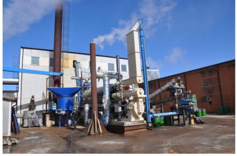
The Torrefaction process takes place in a rotary, tubular reactor which is heated indirectly with flue gases from a biosolids furnace. The flue gas is recovered at two different temperatures, approx.  $350 \,^{\circ}$ C and  $800 \,^{\circ}$ C. The flue gas is mixed in a mixing chamber with a part of the outgoing flue gases from the reactor in order to reach the required temperature.
