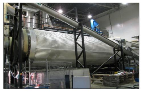
The drying takes place in an advanced energy recovery system based on the combination of a belt dryer and a rotating tubular dryer. The tubular high temp dryer (HT) uses steam as heat source which provides a high drying capacity and an even final dryness in the material. The hot and humid ventilation gas from the HT dryer together with the flue gas from the biofuel combustion are condensed. The heat is then recovered for usage in the
