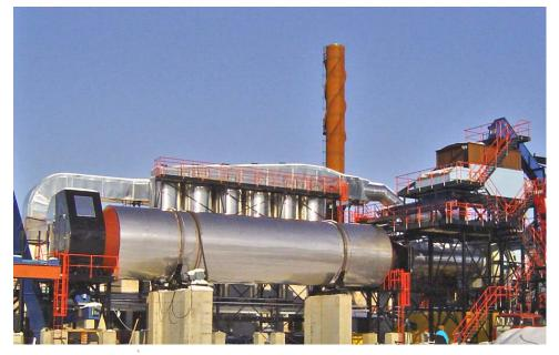
This direct system for drying of biofuels is a simple and robust system with a high degree of energy utilisation (exhaust gases are cooled in the dryer to approx. 80°C).
