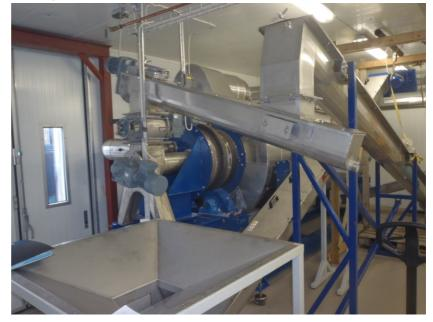
The drying takes place in a rotating tubular dryer which is heated indirectly by flue gases.
