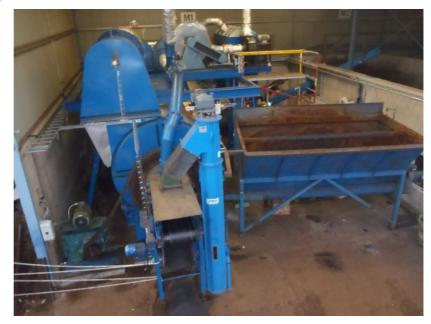
The drying takes place in a rotary tubular dryer which is heated indirectly by flue gases.
